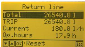
Total: Reset the total amount of the fuel which has passed through the return line since commissioning. This value must be reset in case the flow meter was changed.
