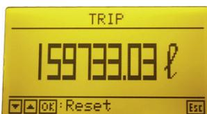
This picture shows the consumption of the Engine since the last reset.
