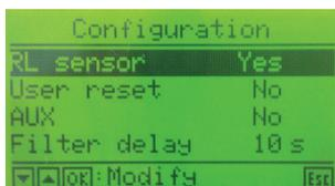
RL flow meter: Is a Return flow meter installed? Answer this question according to the measurement you use (differential measurement or direct measurement) Attention: incorrect setting of this parameter will result in wrong consumption calculation.
