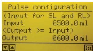
Input value: enter the value of the signal (ml/pulse) which is coming from the flow meter used (see table). This value is used also for the second flow meter (if installed).
