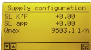
SL KF: Enter the SL K'F-value which you will find on the type plate of the flow meter. This value is to optimize the flow meter performance.
