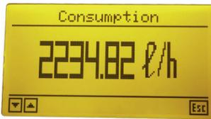
This picture shows the current consumption of the Engine in l/h.
