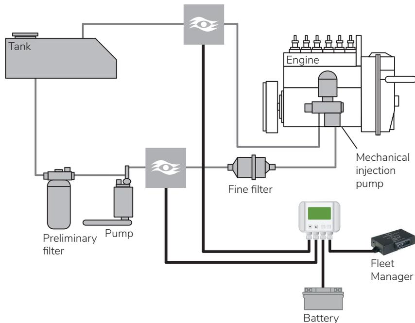
The 2 flow meters are just as an example. Both can be changed with a compact one.
