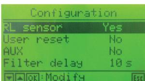
**RL sensor** (flow meter): is a Return Line flow meter installed? (Yes / No)
