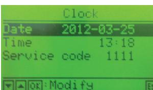
Move the bar over the line you would like to change parameters and press OK. The changeable field will be highlighted for changing.
