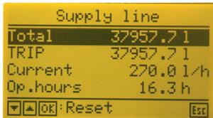
Total: Reset of the total amount of the fuel which has passed through the supply line since commissioning. This value should only be reset in case the flow meter was changed.
