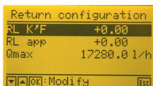
RL cal: Enter the RL K'F-value which you will find on the type plate of the flow meter. This value is to optimize the flow meter performance.
