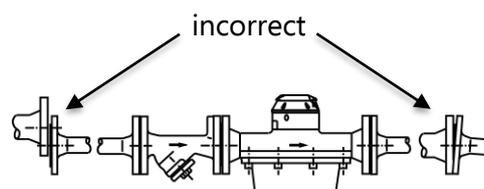
For pipes made of copper or thin-walled steel pipes, the flow meter requires additional fastening. Use appropriate fasteners.
