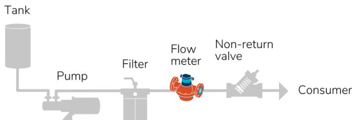
Pressure shocks during operation with the flow meter must be avoided.
