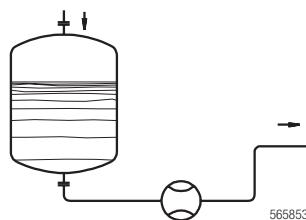
The layout of piping must ensure that the meter, in operating condition, is filled with liquid at all time and that no inclusions of air or gas may occur. The quantities consumed by all the users must be registered by the meter.
